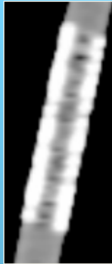
Stationary 4-mm stainless steel stent in a contrast-filled tube scanned using 0.5-mm detector width.
