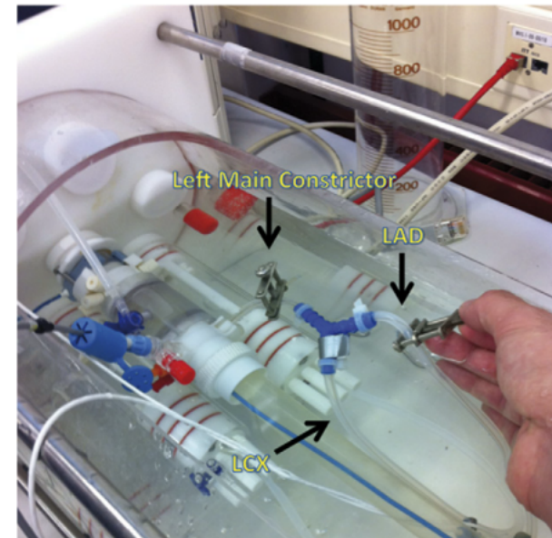
Figure 1. In Vitro Model of the Coronary Circulation
